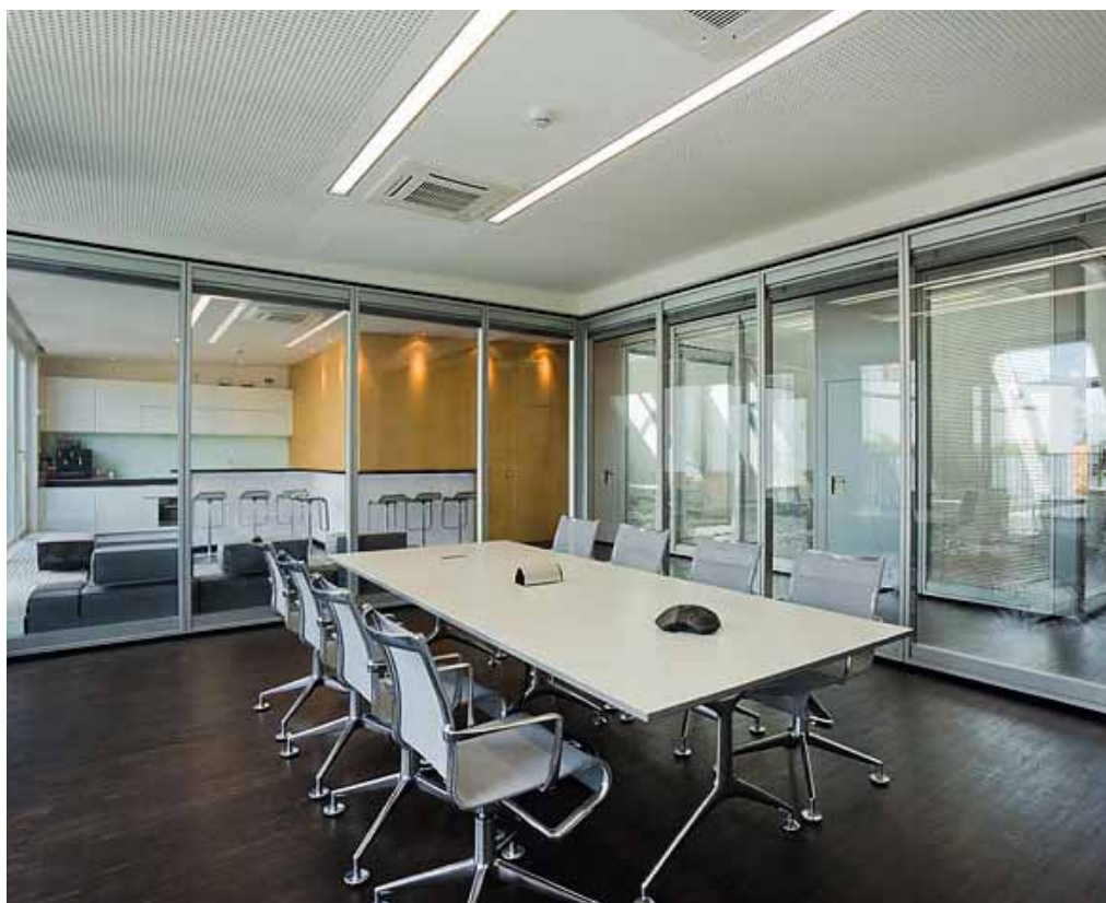
Transparent rooms with a high sound reduction index of up to RW50 decibels (laboratory value measured in accordance with EN 20140) can be created or removed quickly and with a minimum of effort.
